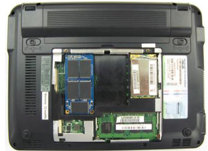
Figure 3: Installing the New SSD
